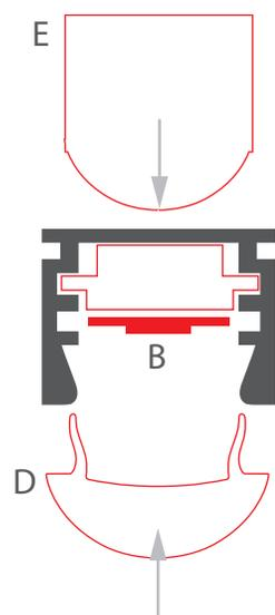
**4. NOTE!** The LED insert can be mounted in five different positions. It is also possible to attach the LED strip directly to the bottom of the extrusion. The smaller the distance between the LED strip and the cover, the wider the light angle.
