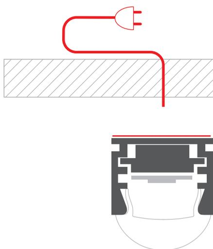
**6.** Attach the extrusion (A) to the surface.
