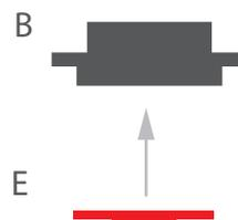
**3.** Slide the LED insert (B) into a selected channel, insert the cover (D) and end caps (E).
