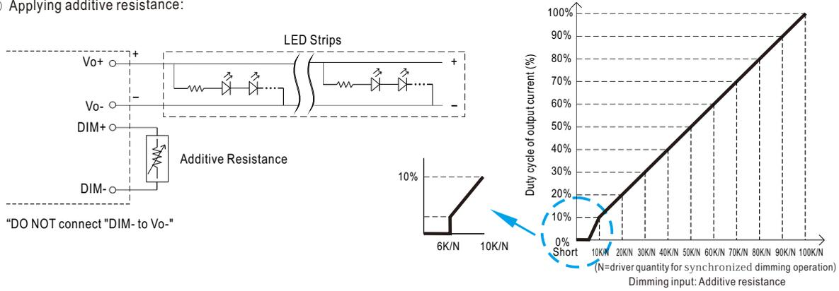
Note : 1. Min. duty cycle of output current is about 0.15%, and the dimming input is about  $6K\Omega$  or 0.6VDC, or 10V PWM signal with 6% duty cycle.
