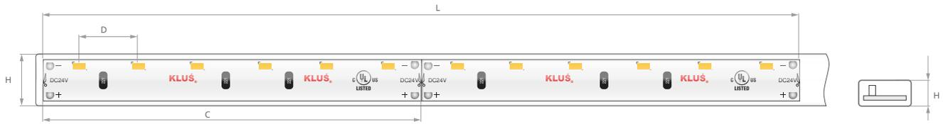
Dimensions: Width [W]: 10 mm | Max run length [L]: 6 m | Cut every [C]: 100 mm | LED spacing [D]: 16.7 mm | Height [H]: 4 mm
