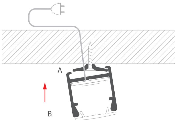
**NOTE!** Unusual disassembly of the extrusion. Move the extrusion (B) horizontally, gently pull one of the sides of the extrusion (B) down, and take the extrusion off the mounting brackets (A).
