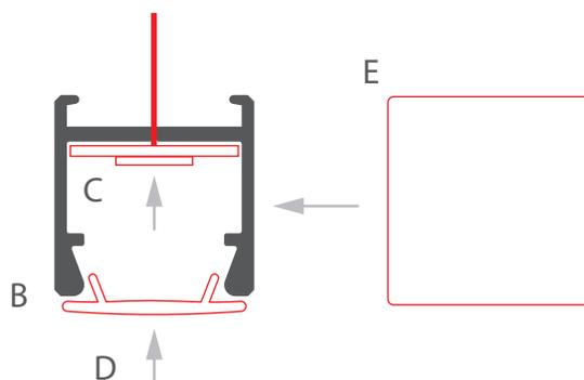
**3.** Connect power to the LED strip and mount the extrusion (B) in the mounting brackets (A).
