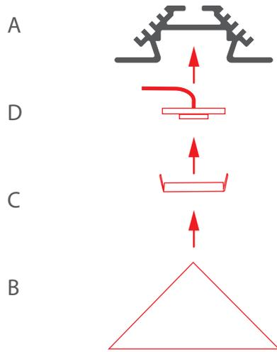
**2.** Apply glue to the mounting surface. Connect power and mount the extrusion.
