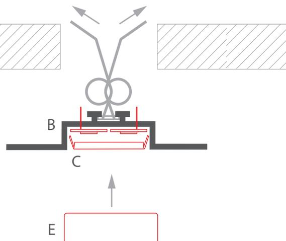
**3.** Place the extrusion in the groove and connect the LED power cable.
