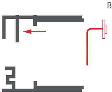
**3.** Degrease the glass and attach the upper part of the extrusion (B).
