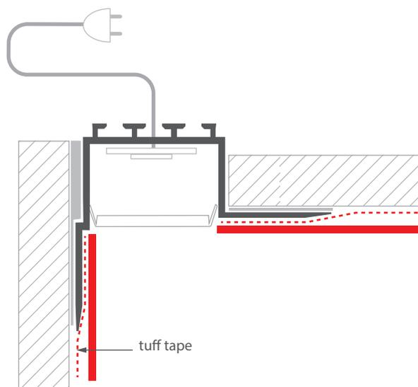
**5.** Slide a sharp tool between the extrusion and the insert (on both sides of the insert) to cut off the layer of plaster and paint from the insert.
