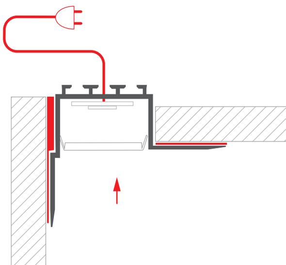
**4.** Apply a layer of plaster to the ceiling, wall and fixture, sand and paint the surface.
