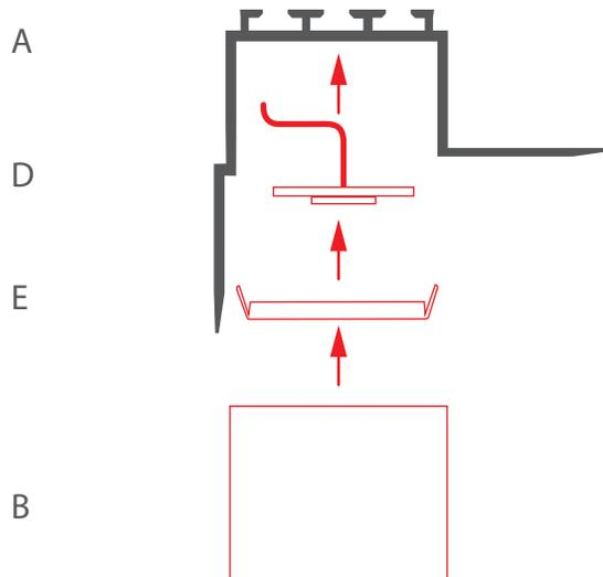
**3.** Glue the fixture to the wall and ceiling using the adhesive and attach the power cable to the power supply.
