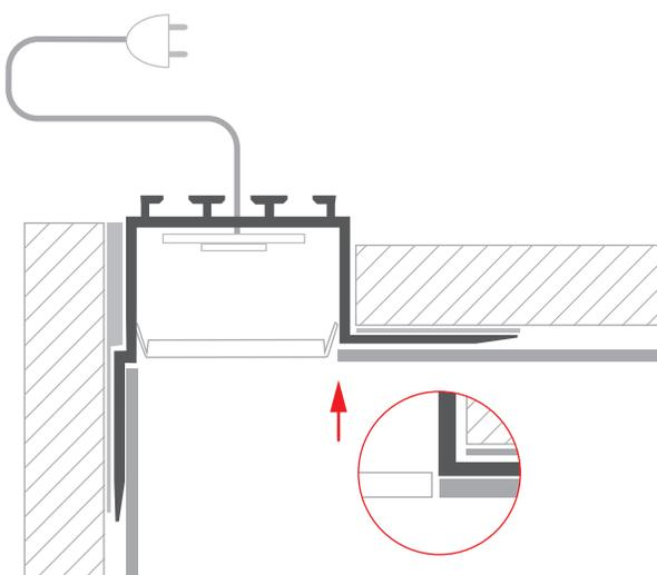
**6.** Remove the protective insert (D) and insert the proper cover (C).
