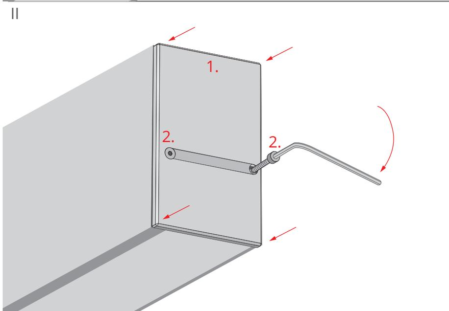
Mount and lock the end cap (1) in the profile by tightening the socket head bolts (2) with an allen wrench.
