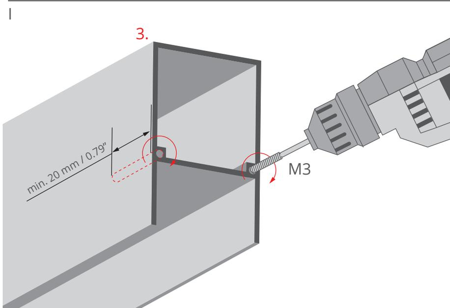
Thread the channels in the profile (3) with a M3 screw tap to a minimum depth of . 20 mm / 0.79"
