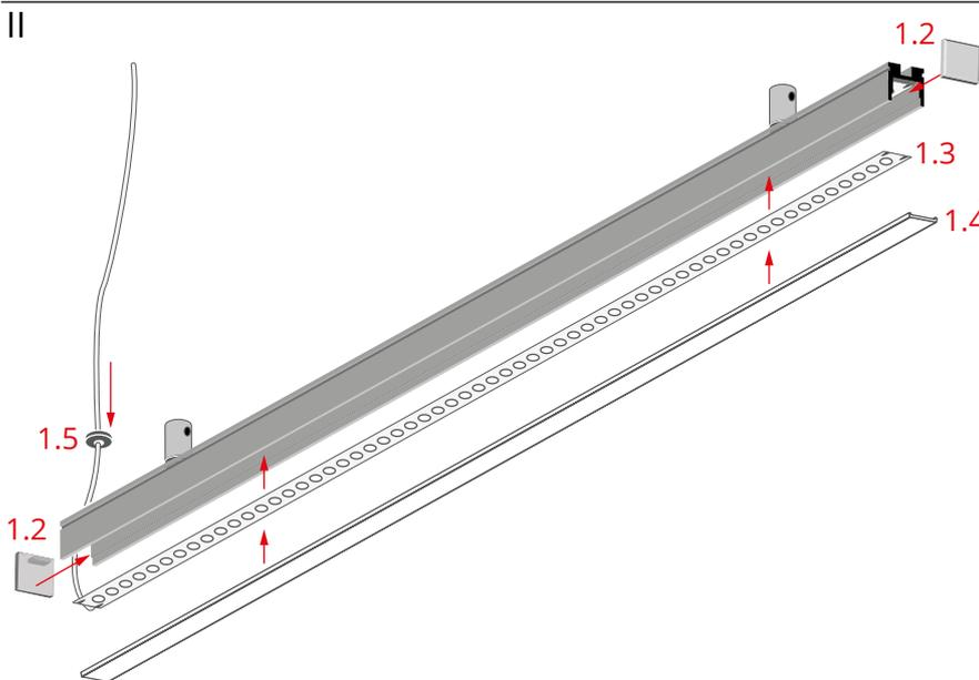
Mount the gland (1.5), in the profile, adhere the LED tape (1.3), and attach the end caps (1.2) and the cover (1.4).
