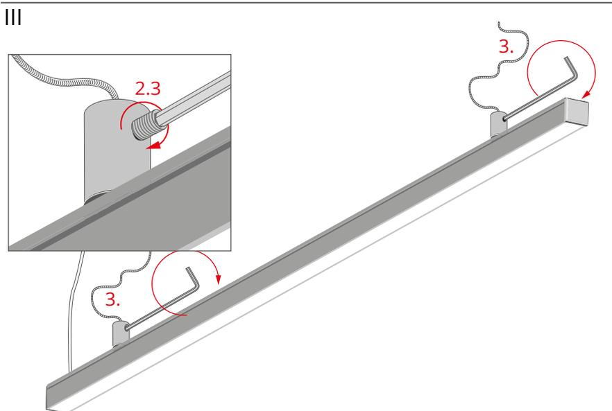
Insert the cables (3) into the heads and lock them by tightening the pressure screws (2.3).
