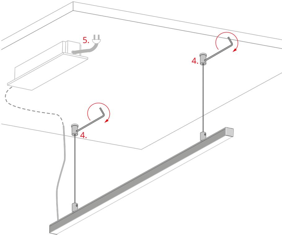
Suspend the lighting fixture from the ceiling fasteners (4) and connect the cable to the 12 V / 24 V power supply (5).
