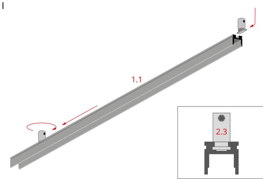
Insert the fasteners into the channel on the back of the profile and lock them by tightening the heads (2.3).
