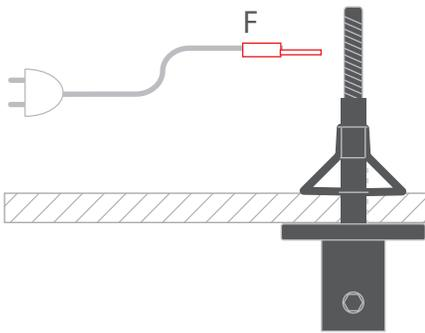
**8.** Thread the lower nut (E) onto the rod, electrical connector (F) and finally the upper nut (G) tightly so that the electrical connector does not move.
