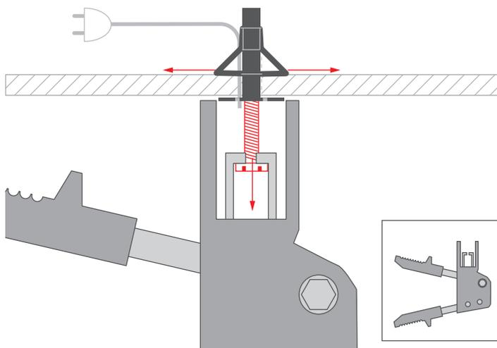
**4.** Remove the screw from the anchor.
