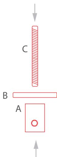
**6.** Mount all in the anchor so that the masking cover will fit tightly against the drywall.
