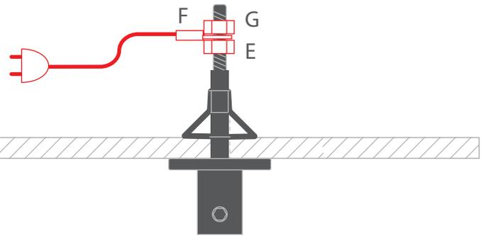
**9.** Mount threaded rod from the fixture into the head. Block the rod by tightening the allen screw with the allen key
