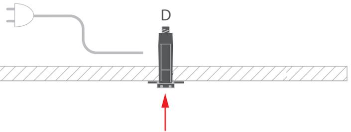
**3.** Pull the screw with dedicated hollow wall anchor setting tool to expand the anchor and secure it in the drywall.
