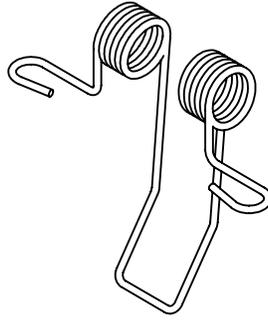
**1.** Insert the spring into the channels in the extrusion.
