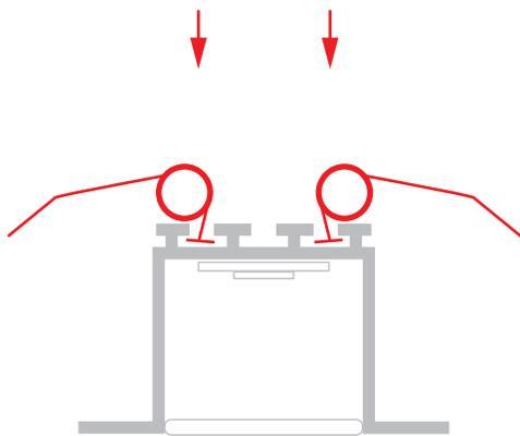
**2.** Insert the extrusion in the groove bending the spring arms towards each other.
