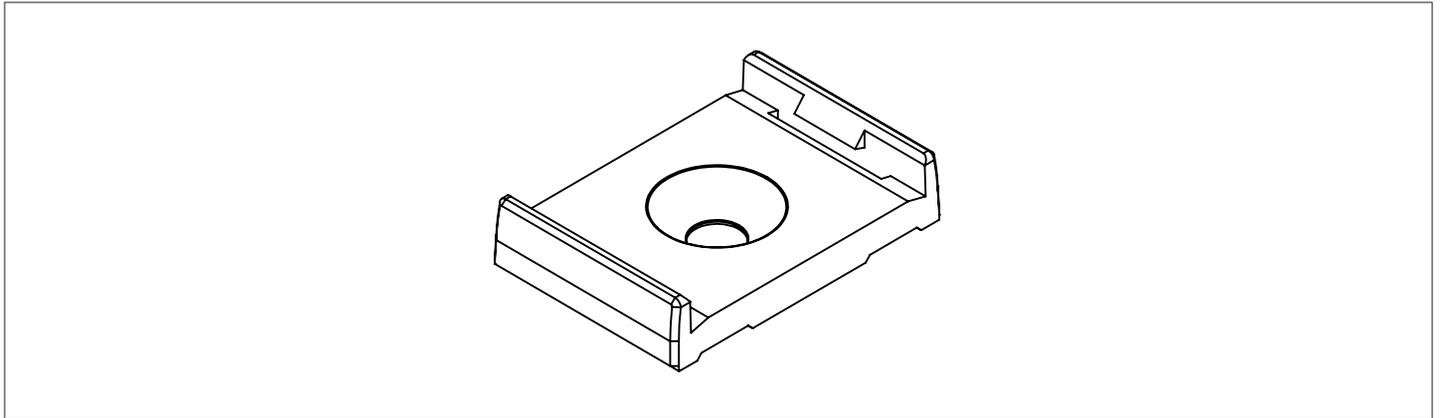
**1.** Attach the mounting bracket to the surface with screws.
