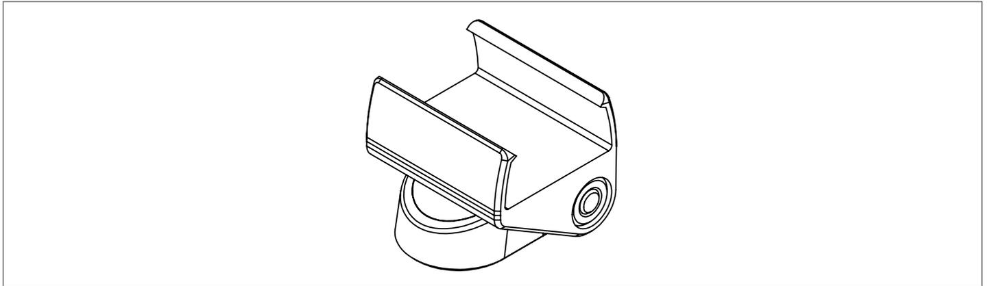
**1.** Remove the masking cover covering the screw hole and attach the mounting bracket to the surface using screws.
