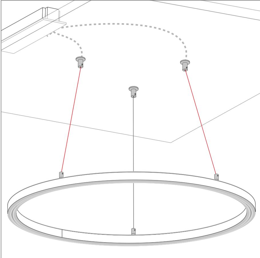
a) Power through the suspension system - p. 2
