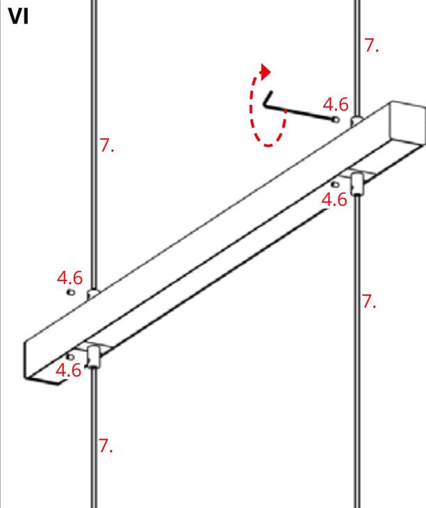
After tightening the fastener's pressure screw, do not tighten or unscrew its head! This will damage the connector.
