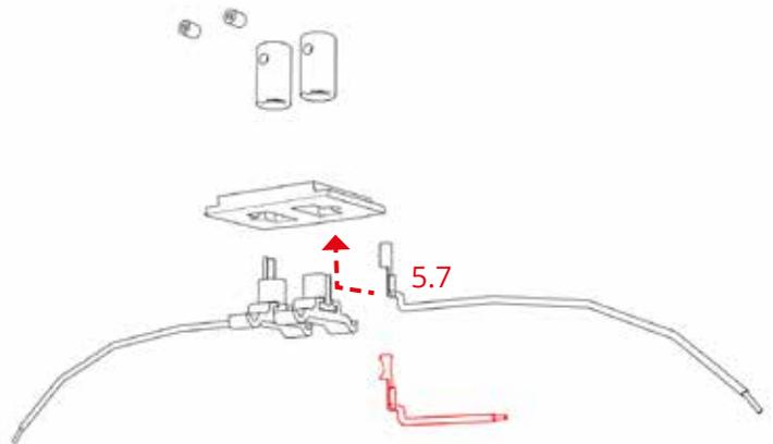
In case of damaged fastener's connector, unfold it for parts and replace damaged item.
