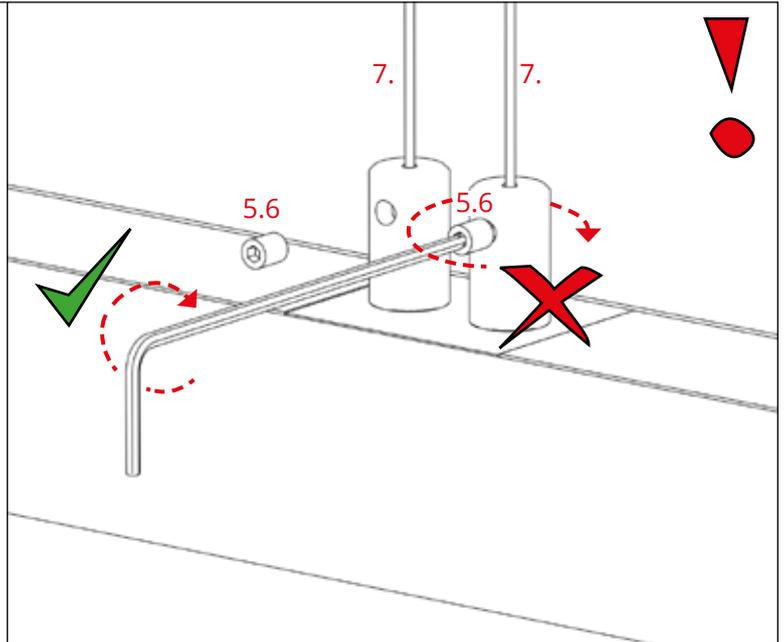
After tightening the fastener's pressure screw, do not tighten or unscrew its head! This will damage the connector.
