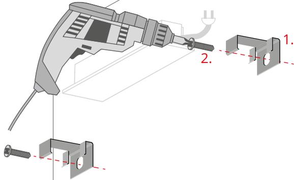
Attach the mounting bracket (1) to the surface with appropriate screws for the surface (2) (not provided).
