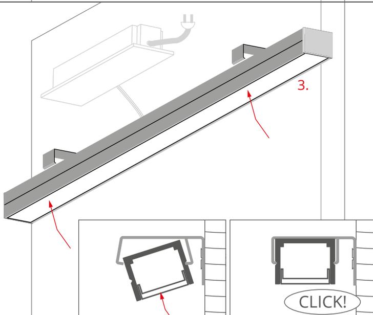
Snap the lighting fixture (3) into the brackets.
