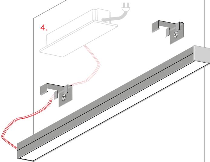
Feed the power cable from the fixture to the power supply (4).
