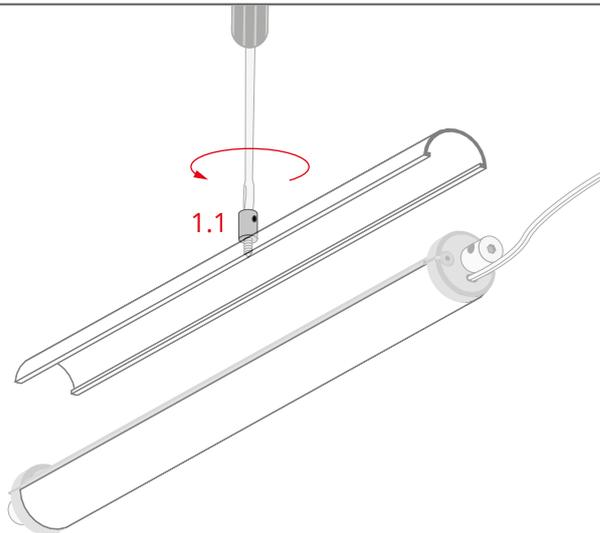
Screw the fastener body (1.1) into the pre-drilled hole.
