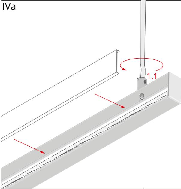
Screw the fastener body (1.1) into the pre-drilled hole.
