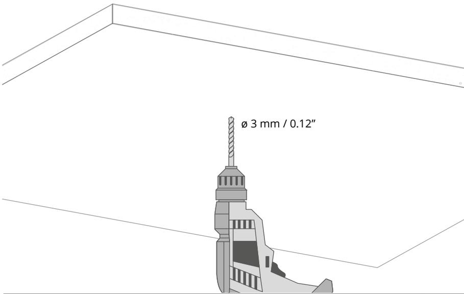
Drill a 3 mm / 0.12" hole in the ceiling. In case of metal surfaces, it should be 3,5 mm / 0.14" hole.
