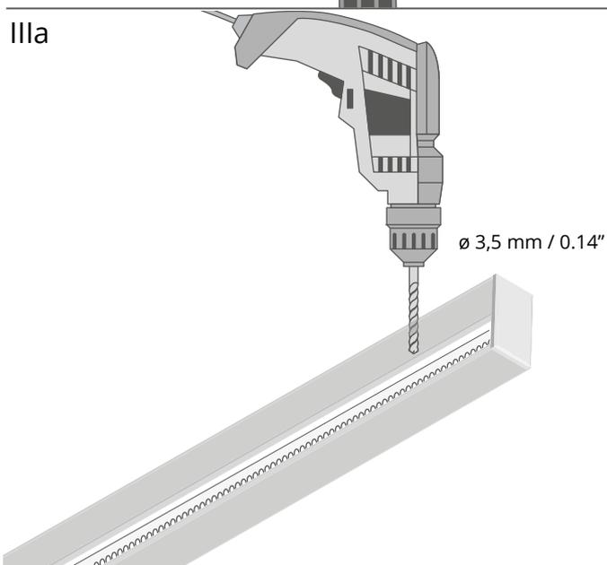
Drill a hole in the profile's wall. Width of the hole for the aluminium surface should be 3,5 mm / 0.14".
