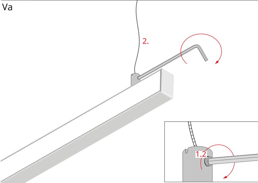
Insert the wire (2) to the hole in the fastener body and tighten the pressure screw (1.2) with an allen wrench.
