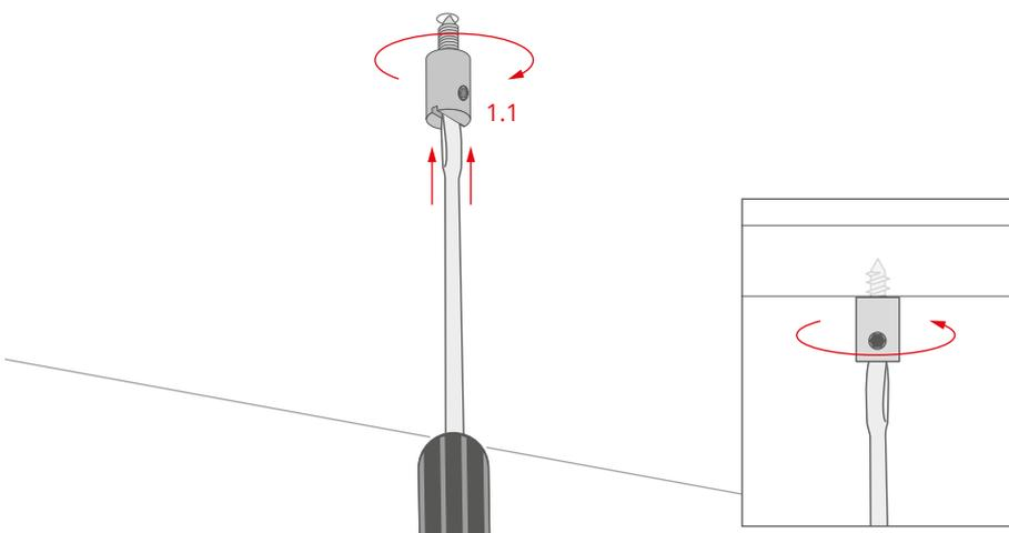
Screw the fastener body (1.1) into the pre-drilled hole.
