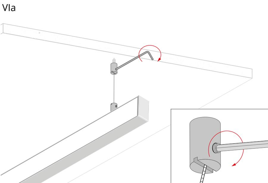
Suspend the fixture on the ceiling fastener, repeating the procedure from chapter Va.
