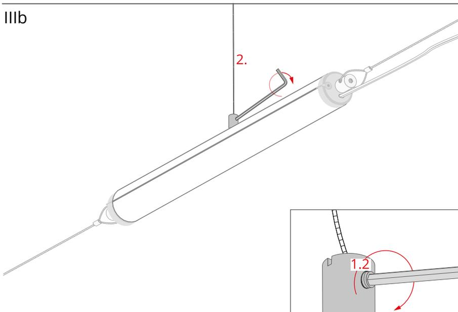
Insert the wire (2) to the hole in the fastener body and tighten the pressure screw (1.2) with an allen wrench.
