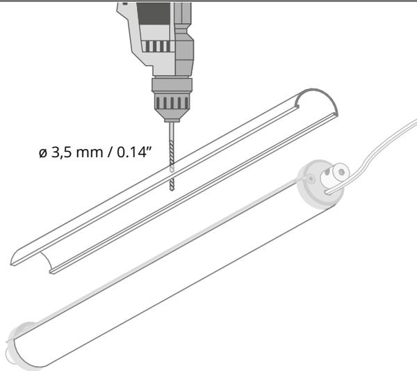
Drill a 3 mm / 0.12" hole in the fixture's cover.
