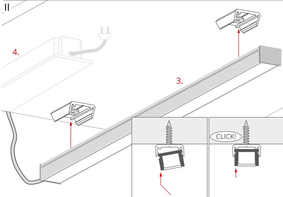
Connect the fixture (3) to the power supply (4) and mount it in the brackets.
