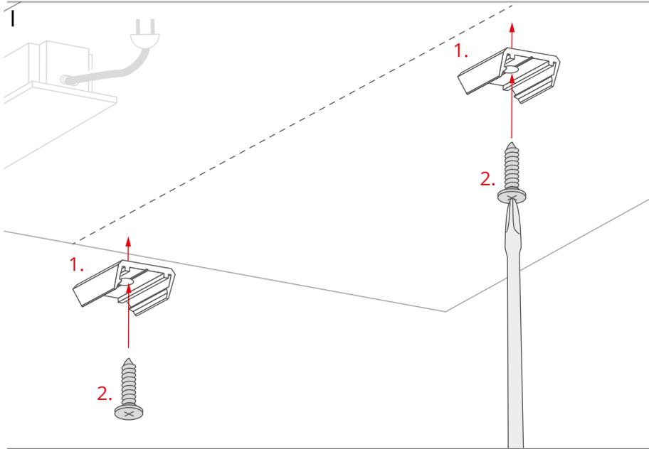
Screw the K-10 mounting brackets (1) to the surface with the use of screws (2). the brackets must be aligned in a straight line.
