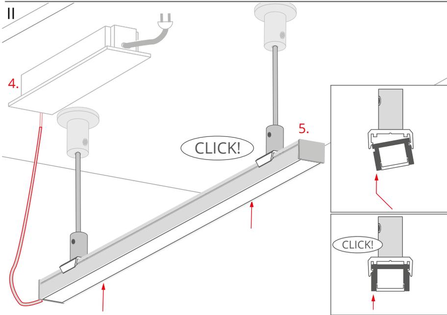
Connect the lighting fixture (5) to the 12 V / 24 V power supply (4) and snap it in the fasteners.
