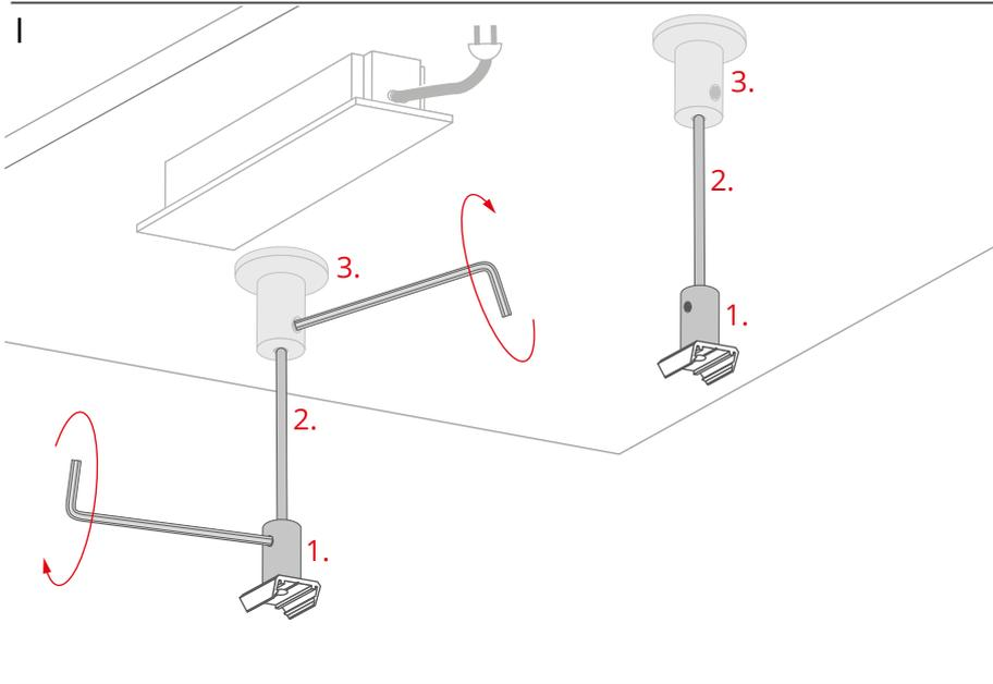
Mount the fasteners (1) on the rods (2) and on the wall fasteners (3).
