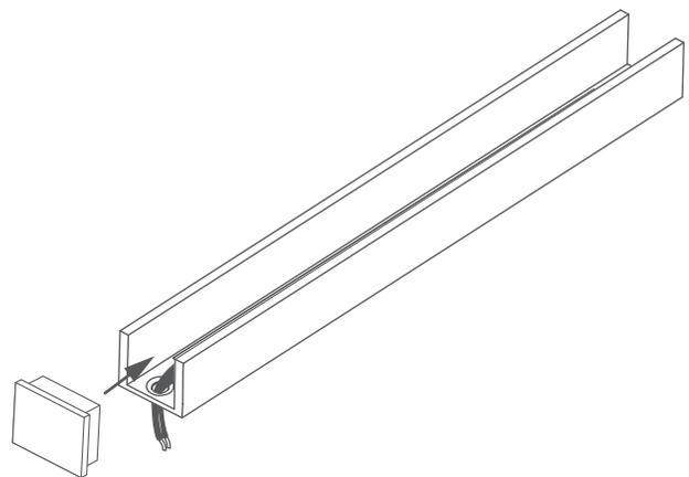
**OPTIONALLY:** It is recommended to attach the end caps to the extrusion with use of glue.
