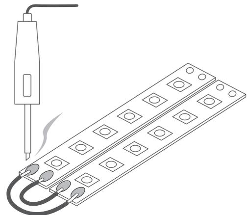
**OPTIONALLY:** The LED strips can also be connected using a system of LED strip connectors. More information at [www.klusdesign.eu](http://www.klusdesign.eu)
