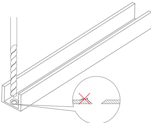
**NOTE!** Some extrusions feature one or more special grooves that make it easier to start drilling.
