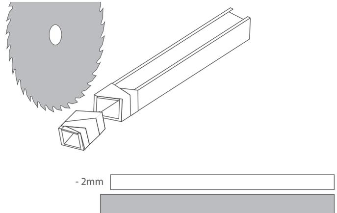
**NOTE!** Low precision cutting of the extrusion and cover can be done with a hand saw, however, uneven, jagged edges will remain, and the covers may break.
