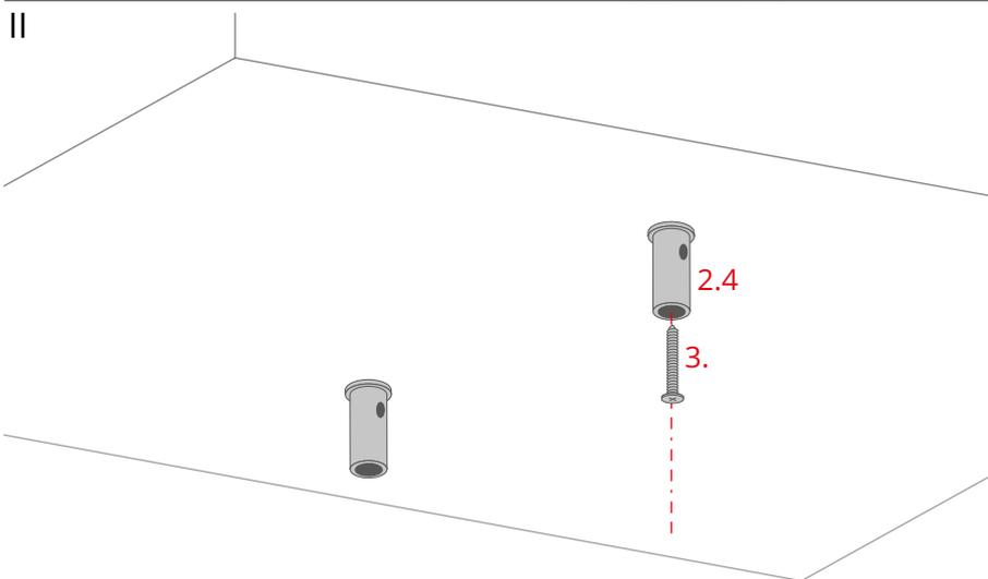
Screw the ceiling brackets (2.4) with appropriate bolts (3).
