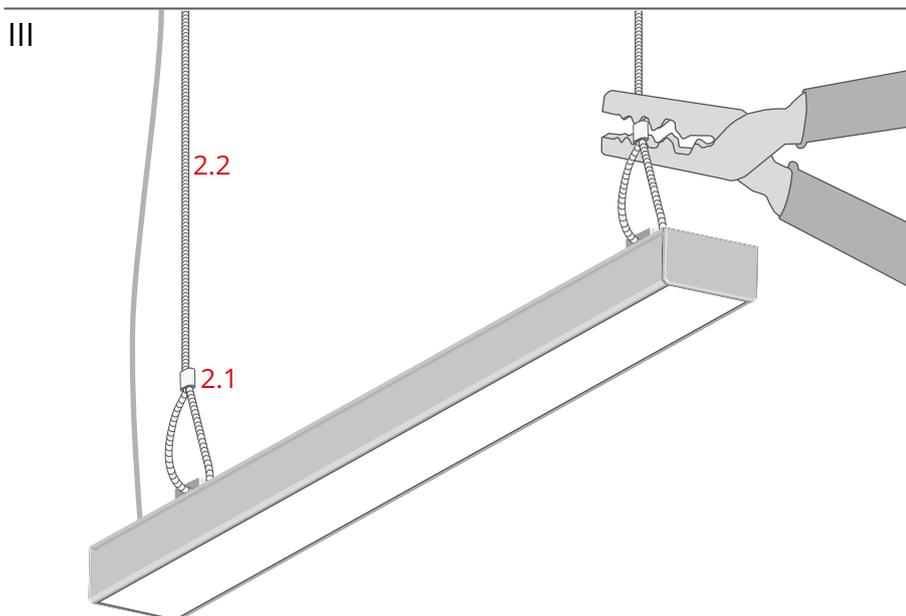
Attach the wires (2.2) to the hangers of the lighting fixture and secure them with crimp sleeves (2.1).
