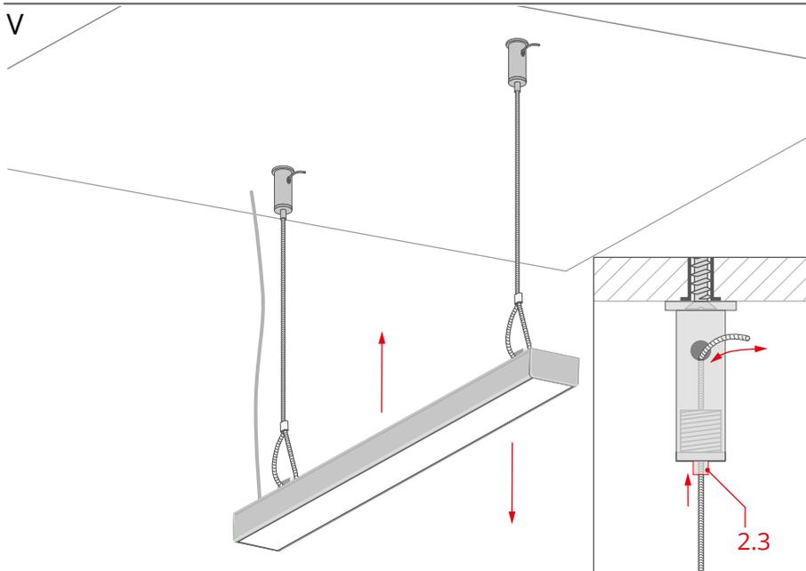
Adjust the position of the suspended fixture using the blocks (2.3).
