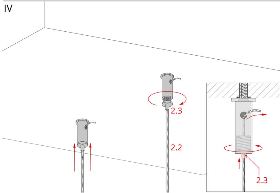
Feed the wires (2.2) through the blocks (2.3) and through the hole in the ceiling bracket. Screw the wire blocks.
