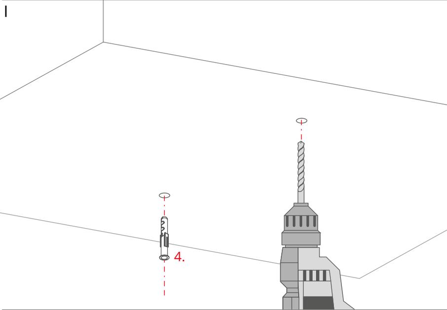
Prepare holes in the ceiling using appropriate wall anchors (4).
