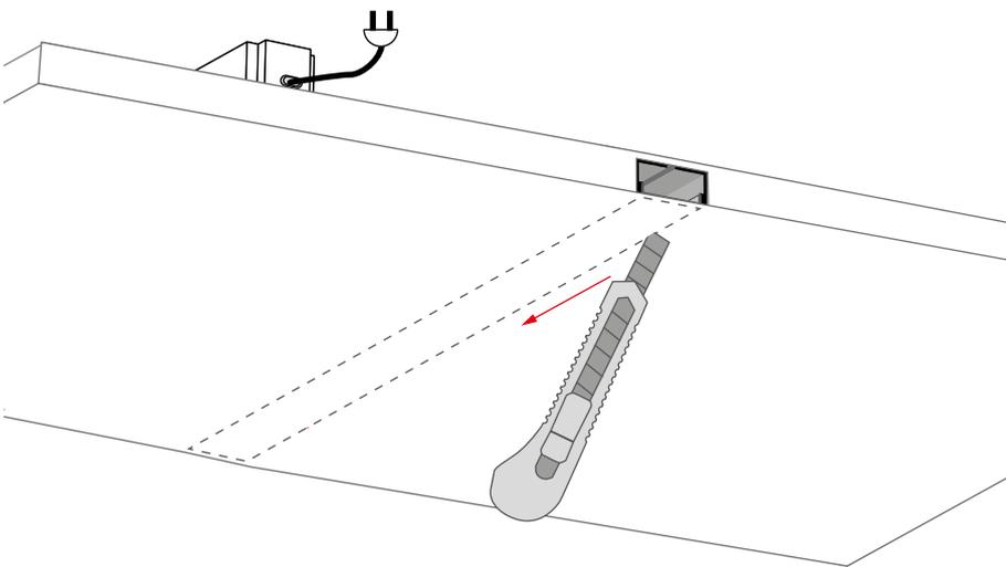
Cut layers of paint and plaster at the junction of the aluminum edge of the profile and the protective insert.
