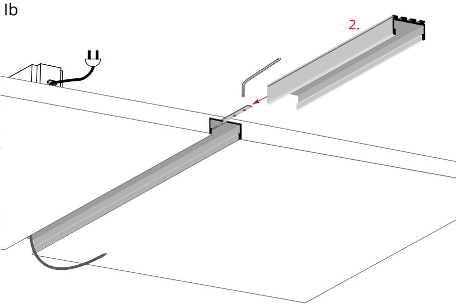
Slide the internal channel of the GIZA-LL profile (2) onto the protruding part of the connector. Finally tighten the connector screws with the Allen key.
