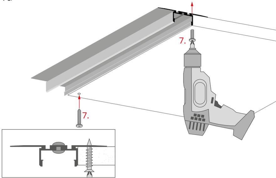
Insert the drywall screws (7) in the pre-drilled holes and screw the profile flange to the board.
