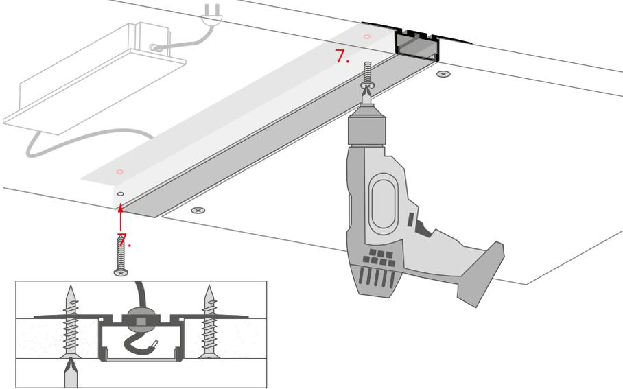
Insert the drywall screws (7) in the newly drilled holes and screw the second flange of the profile to the board.
