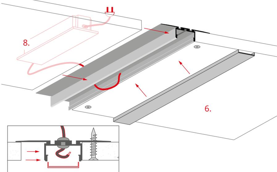
Route the cable from the power supply (8) through the gland.
