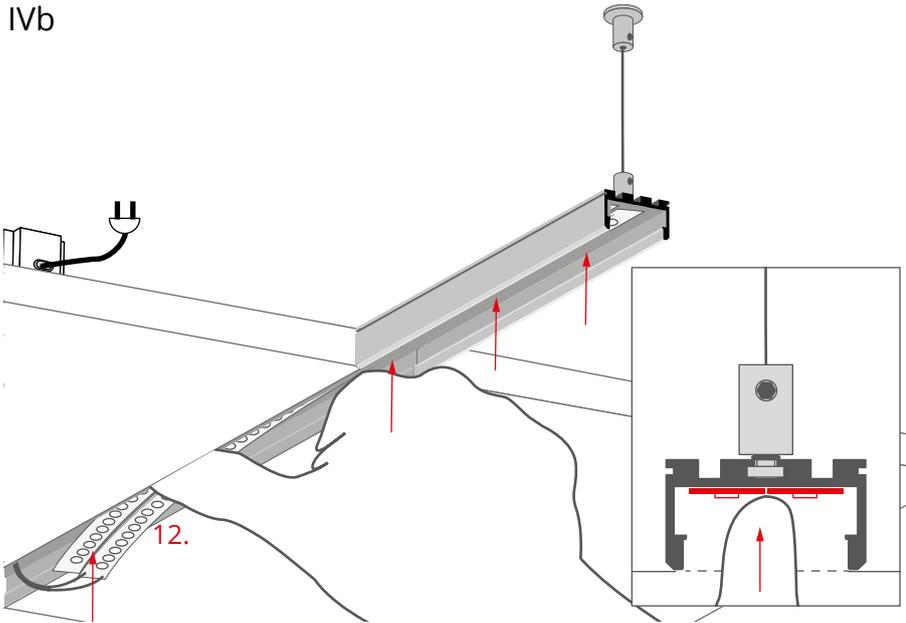
Connect the LED tapes to the power supply.
