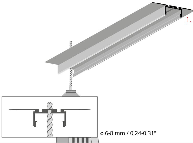
Drill a hole for the power cable in the GIZA-LL-T (1) profile.
