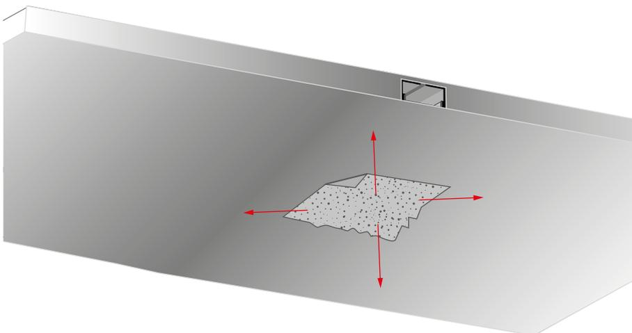
After the plaster has dried, sand the surface with sandpaper.
