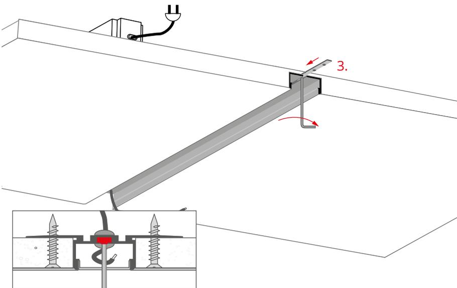
Insert the connector (3) into the channel inside the profile and tighten the locking bolts with an Allen key.
