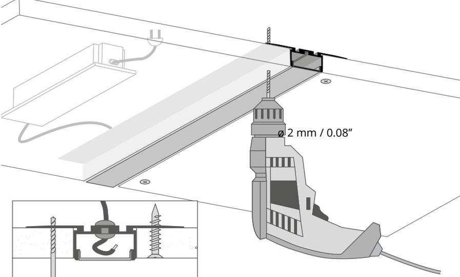
Drill holes in the second board and the profile's flange.
