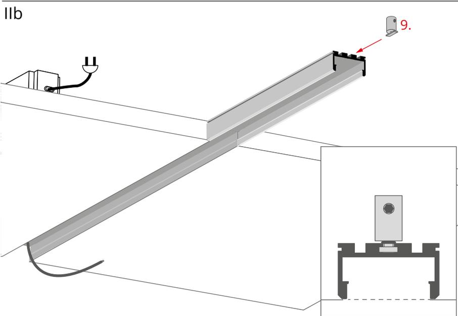
Insert the fastener (9) into the top channel of the profile.
