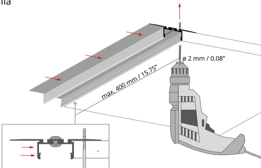
Place the profile on the edge of the drywall board and drill holes through the board and the profile's flange.
