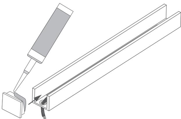
**OPTIONALLY:** Power cables can be run through the end caps in which case the extrusion does not need to be drilled through.
