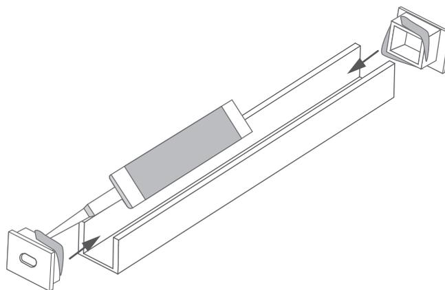
3. Apply a silicone layer to the bottom of the profile and embed the LED strip in it.
